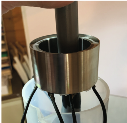
Fig. 6. Plastic tube filled with polypropylene beads being inserted into sensor.
